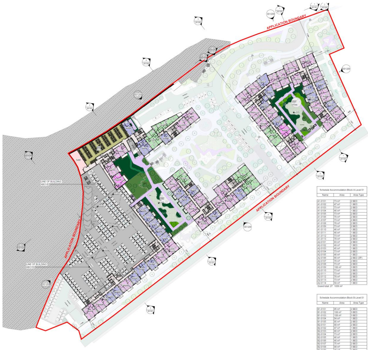
Figure 36.0 Proposed site plan at first-floor level with podium level communal open space at Blocks A, B and C, and first-floor undercroft parking area at Block D
