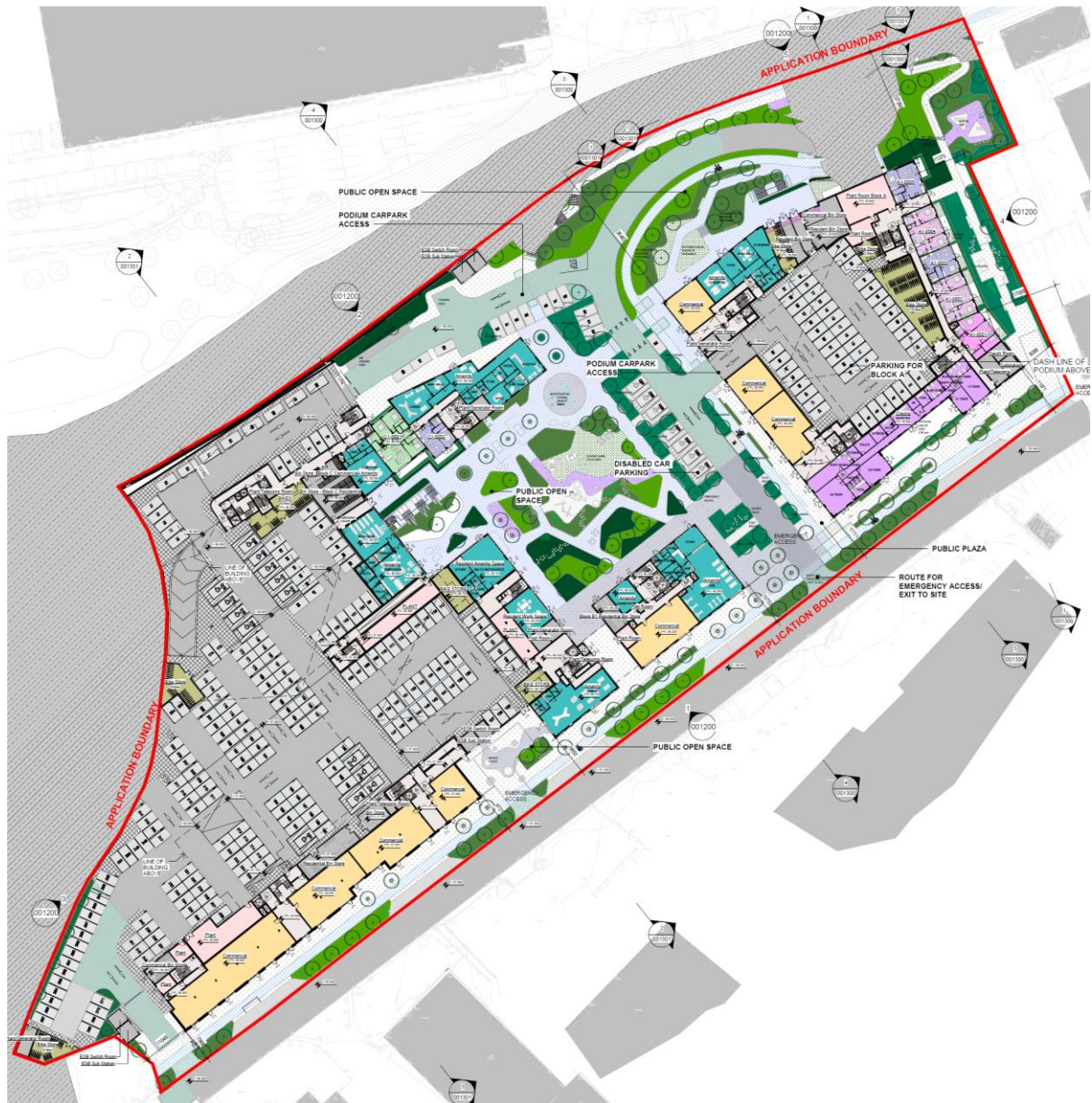
Figure 35.0 Proposed site plan at ground floor level showing public open space and undercroft parking areas
